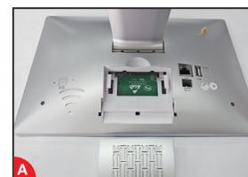
Push down the plate, then open the HDD compartment
