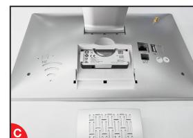
Insert the HDD and ensure HDD SATA port to connect with NVR SATA port
