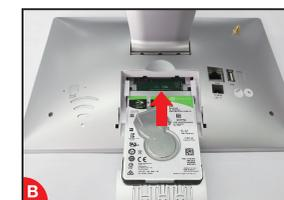
Ensure HDD SATA port on the same position as NVR SATA port before install HDD
