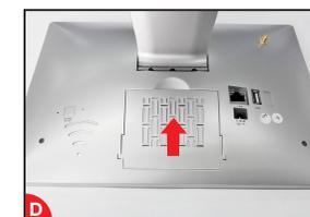
push up the plate and close the HDD compartment
